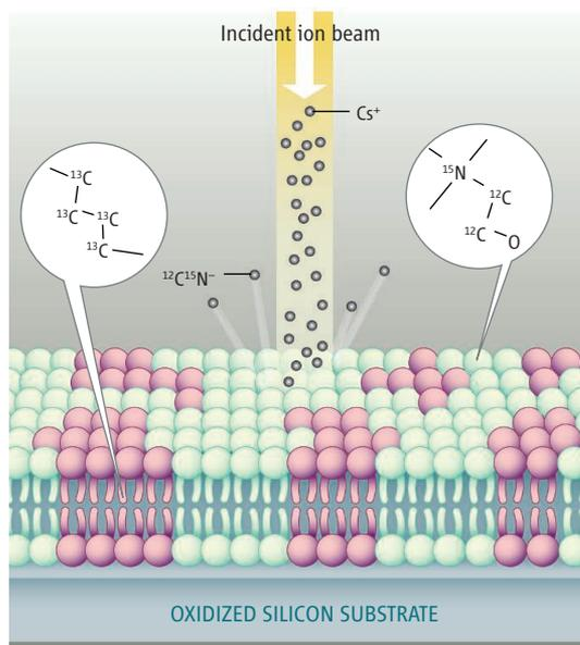
**A detailed look at membrane composition.** In the NanoSIMS experiments reported by Kraft *et al.*, a focused beam of ions bombards the sample, releasing a barrage of small ions that are analyzed with mass spectrometry. By scanning over the bilayer membrane sample, a high-resolution (about 70 to 100 nm) image of its chemical composition is generated.
